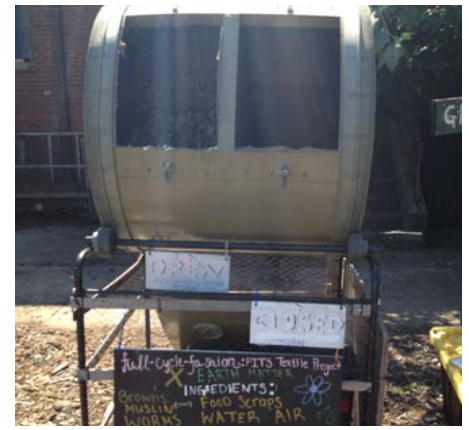
▲ Axle drum tumbler compost bin manufactured by Mantis at the Earth Matter NY demonstration site on Governors Island, New York City. Credit: Institute for Local Self-Reliance
