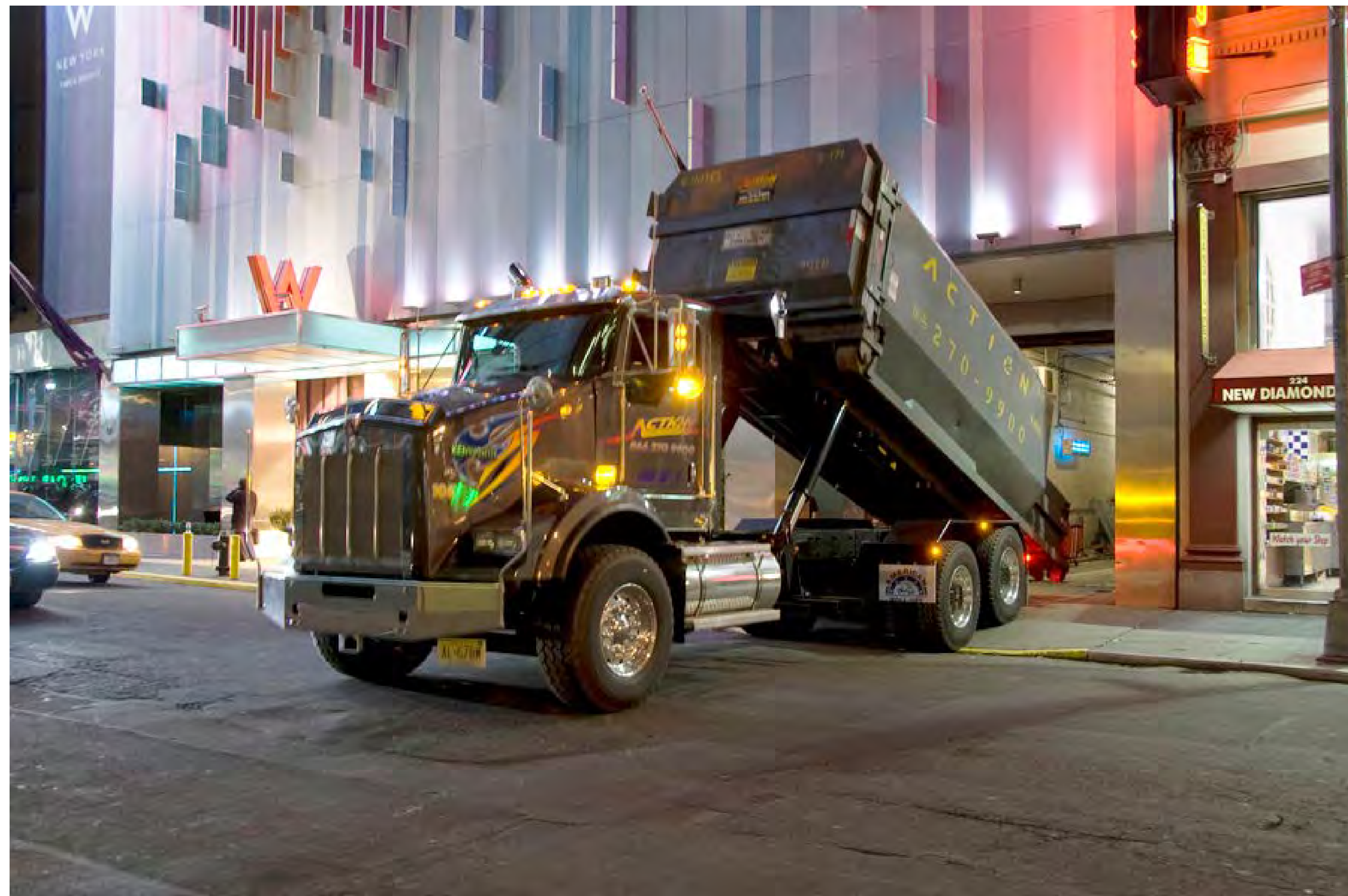
Roll off truck pulling a compactor from a loading dock
