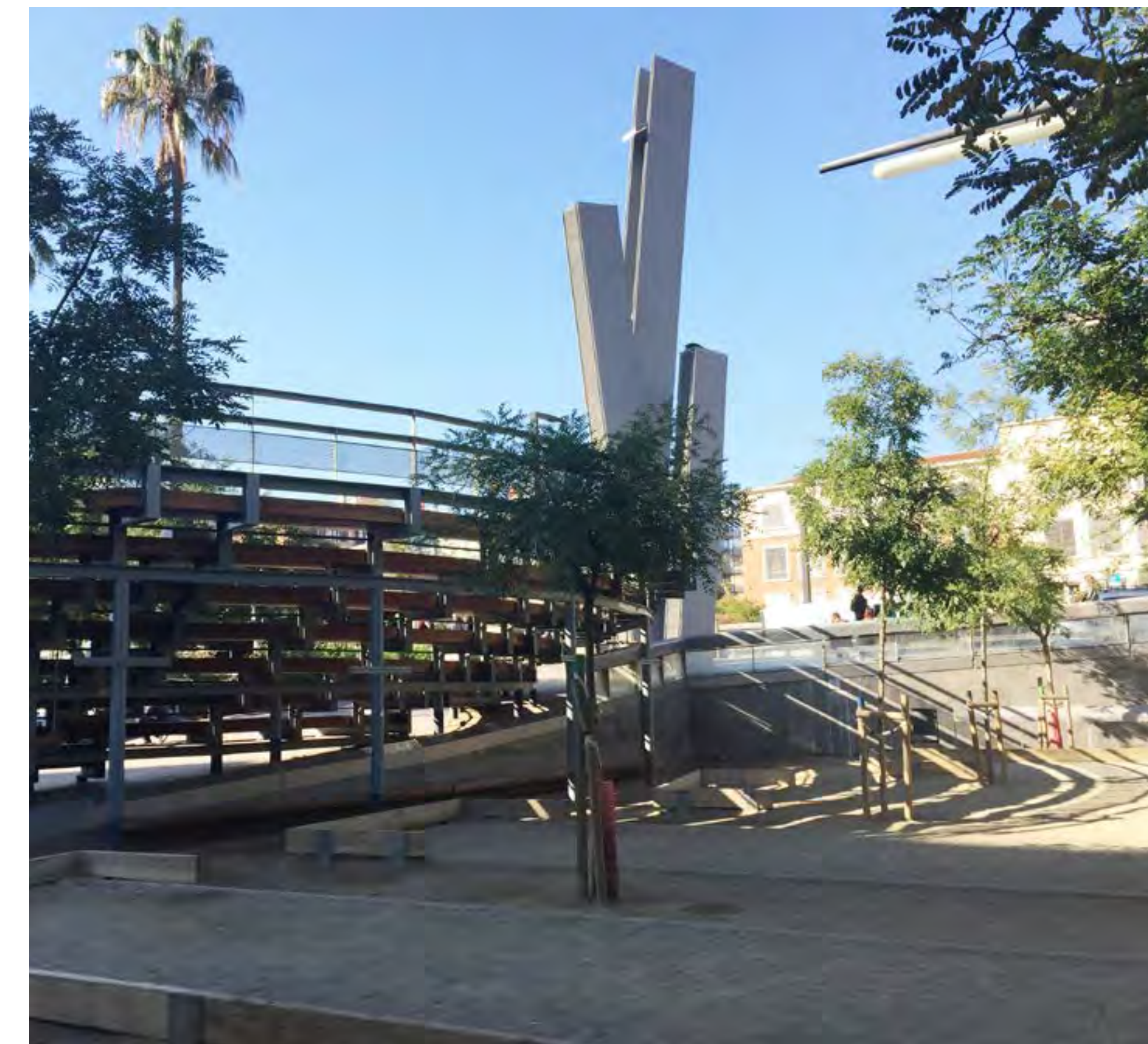
When Plaza Lesseps was built in Barcelona, a pneumatic terminal was inserted under the new plaza to serve the neighborhood; the angular streetlighting is also the stacks for the pneumatic terminal.
