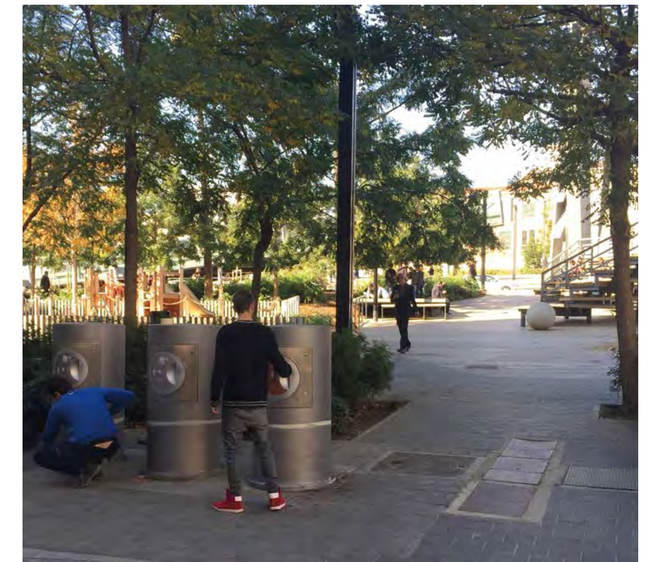
When Plaza Lesseps was built in Barcelona, a pneumatic terminal was inserted under the new plaza to serve the neighborhood; the angular streetlighting is also the stacks for the pneumatic terminal.
