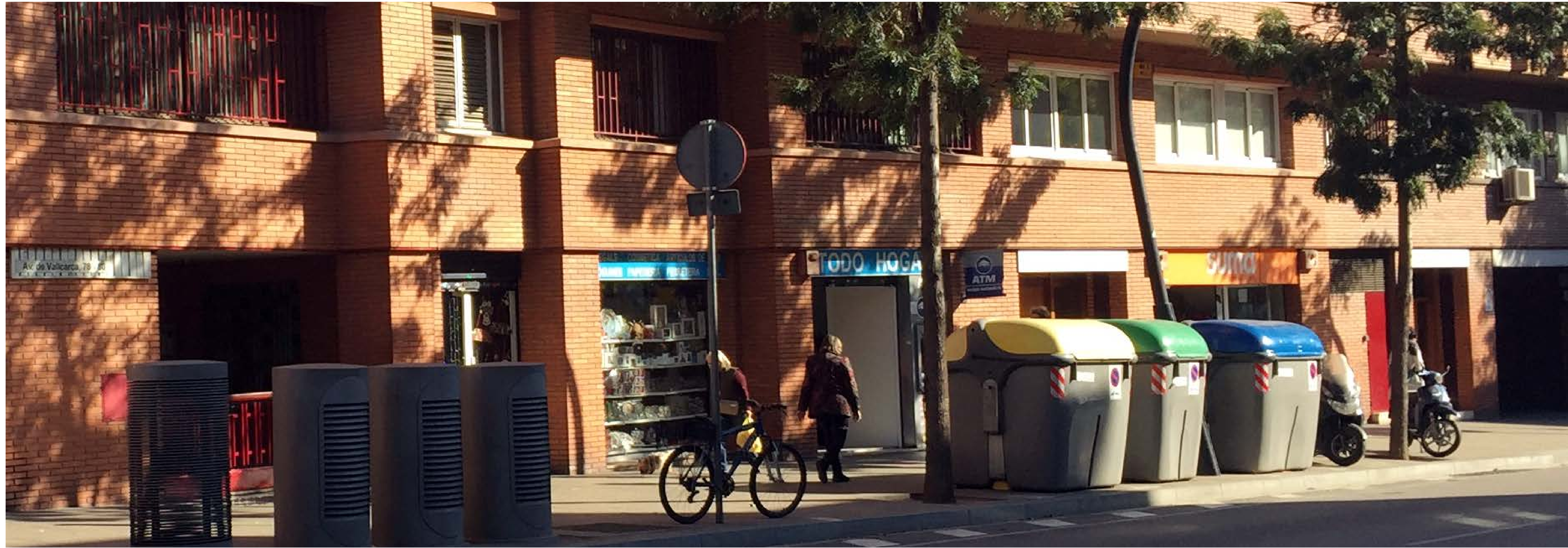
In Barcelona, residents and small businesses bring recycling to shared surface containers (right) and trash and organic waste to pneumatic inlets (left).
