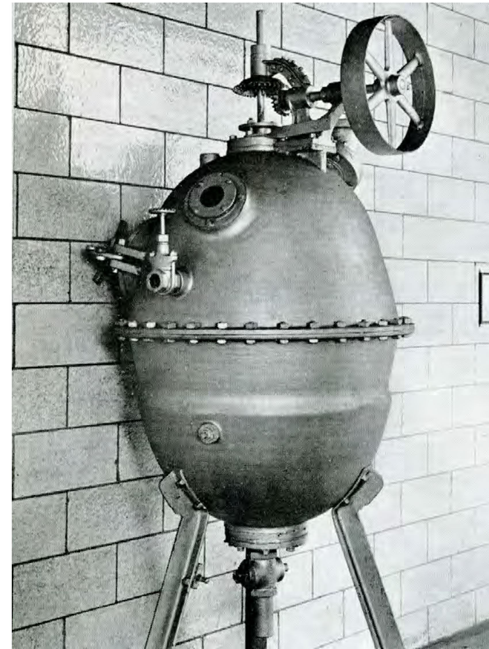
Steam pressure vessel for making bakelite from Leo H. Baekeland's laboratory, 1909
