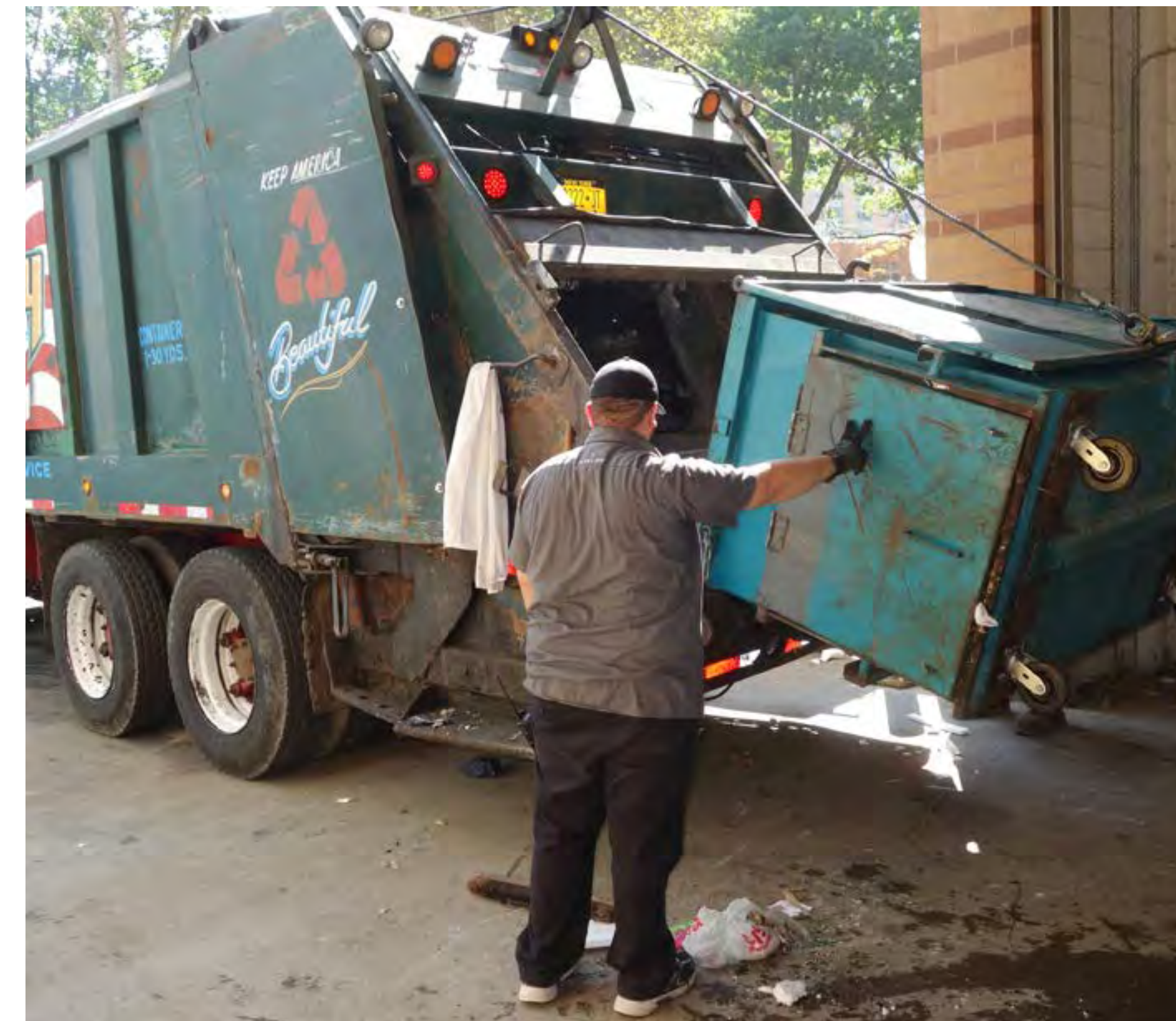
Trash and recycling chutes connect to compactors and 2 cu yd containers which are wheeled to the loading area and emptied into a rear end loader truck.
