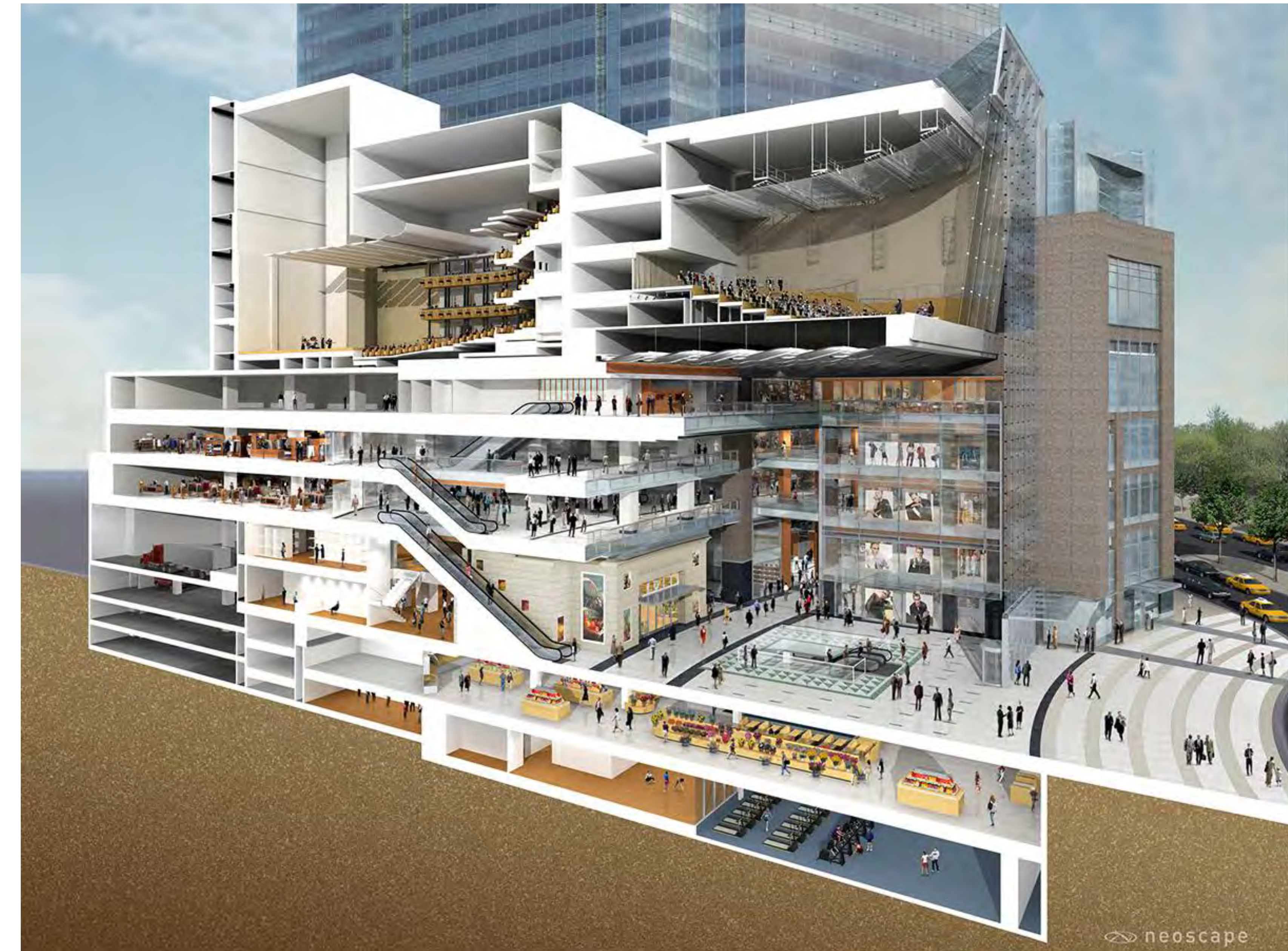
Above: Section perspective of Time Warner Center
