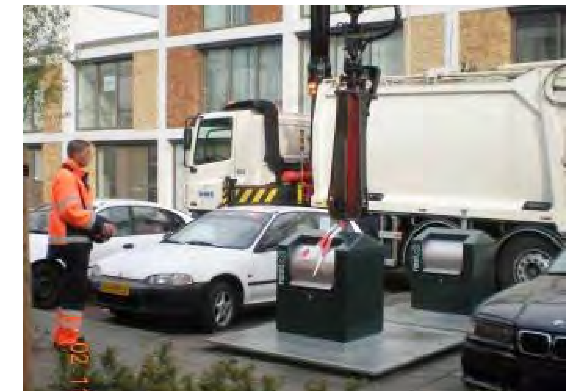
Clockwise from top: Submerged containers installed in a curb extension; truck removing container
