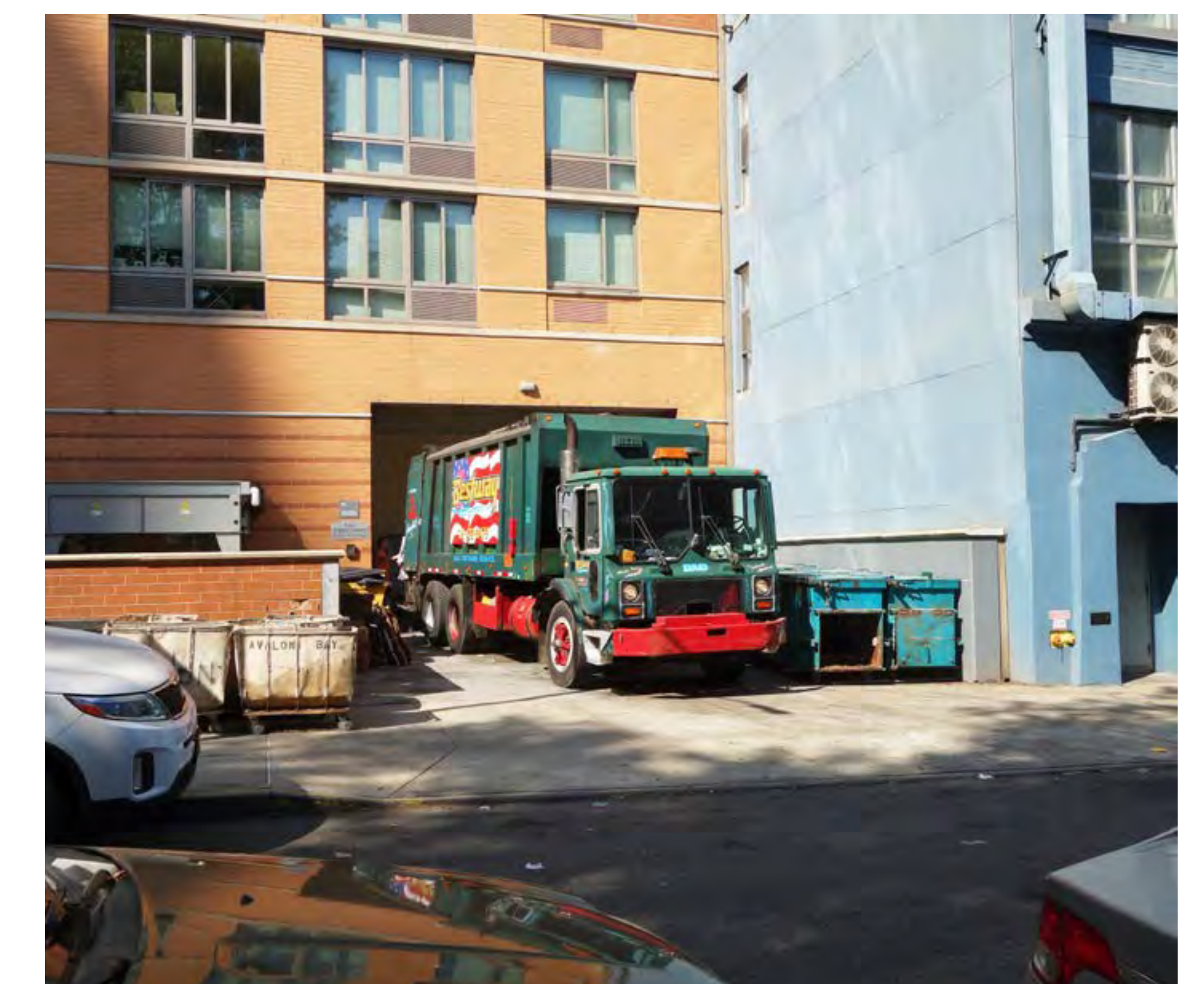
Trash and recycling chutes connect to compactors and 2 cu yd containers which are wheeled to the loading area and emptied into a rear end loader truck.
