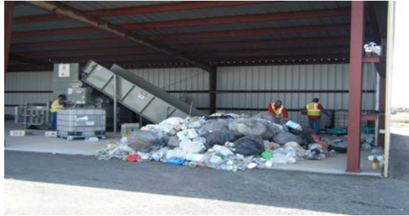
Small Processor: 3,000 square foot processing facility, capable of processing about 4 tons per day.
