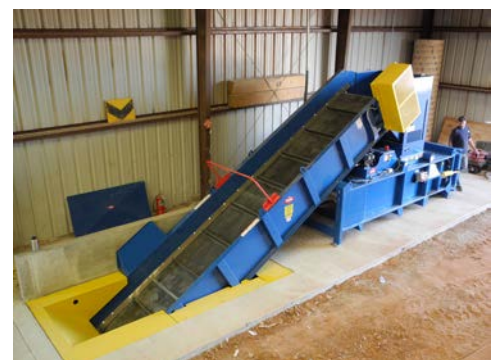
Mid-Size Horizontal Baler Manual Tie in New Mexico Hub
