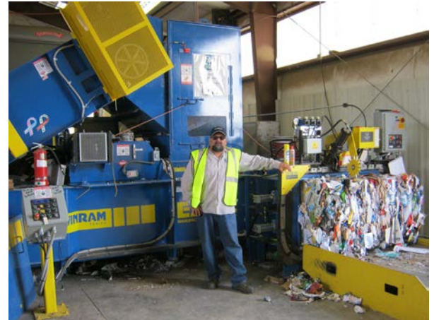
Large Scale Multi-Material Horizontal Baler Auto-Tie at NM Hub
