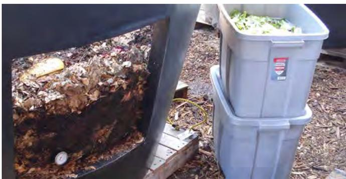
*The Earth Tub is an in-vessel composting system designed specifically for on-site composting of food scraps and other organic matter. Two "tubs" are set up for composting material from select restaurants and office buildings in Old Town Fort Collins. In addition, the City's horticulture center uses two tubs, and a larger scale "Earth Flow" system is used by Colorado State University to compost material from campus dining halls.*
