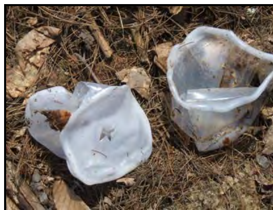
Figure 6--PLA beverage cups, paper cups, paper napkins and bagasse plates, left; PLA beverage cups beginning to degrade after composting 30 days, above.
