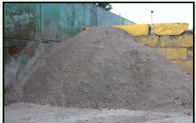
C&D fines replace virgin soil as landfill cover or non-structural fill Material
