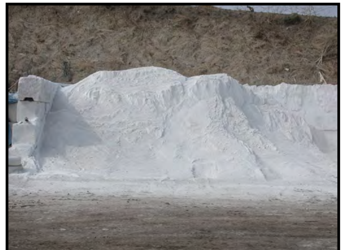
Gypsum separated from drywall is used to make new drywall or as an agricultural product
