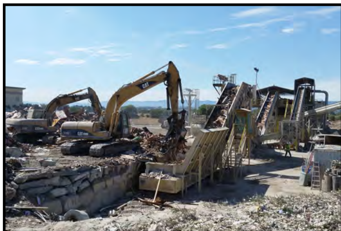
CDRA members use a combination of mechanical equipment and trained employees to separate debris from construction, demotion and renovation projects into marketable commodities
