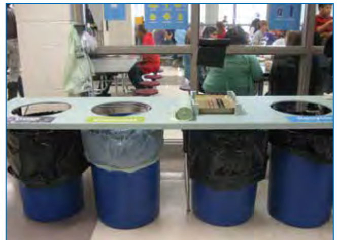
The buildings and grounds department at Wayzata High School made their own sorting tables, complete with varying sized holes to divert bottles and cans away from the larger opening aimed at collecting organics.
