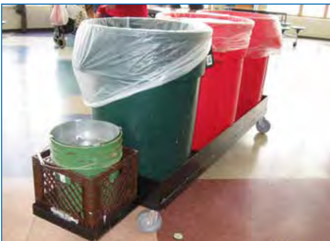
The custodians at Cityview Elementary in Minneapolis helped design a wheeled cart that holds three barrels and a bucket; notice the strainer top on the bucket which allows liquid waste to be safely disposed of down the sink.
