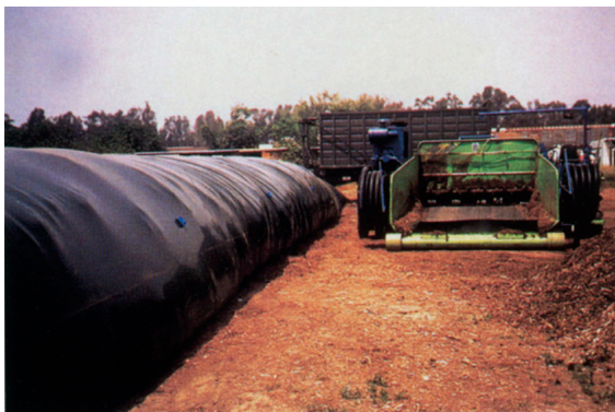
PHOTO 1f "Ag-bag" composting system ( compliments of Ag-bag )
