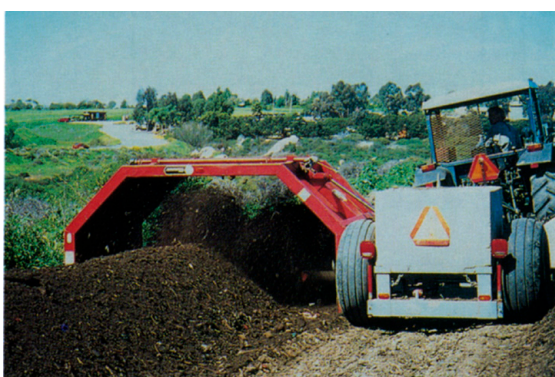
PHOTO 1c Small one-pass windrow turner (California) ( Robert Rynk )
