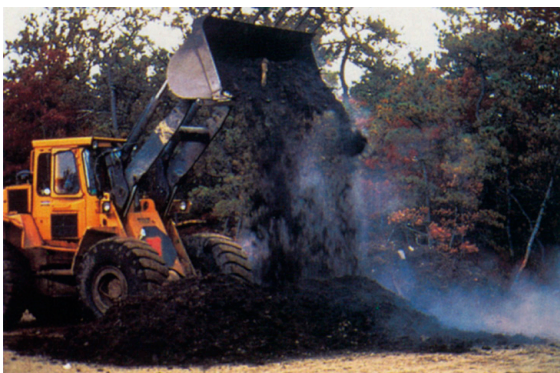
PHOTO 1a Loader lifting and turning ( Bruce Fulford )
