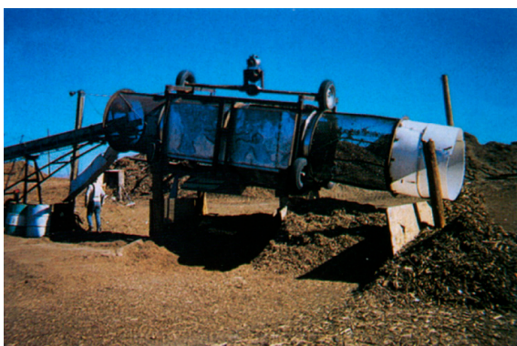
PHOTO 1-4 Homemade trommel screen (Canada) (Robert Rynk)
