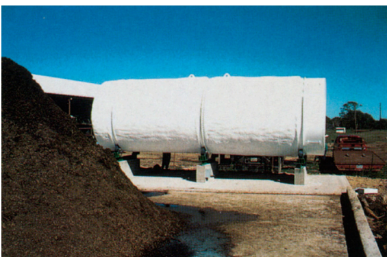
PHOTO 1g Rotating drum vessel on a dairy (Texas) ( Don Cawthon )
