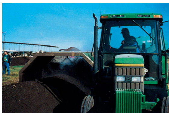
PHOTO 3-1 Moisture addition while turning at a dairy (Texas) (Robert Rynk)
